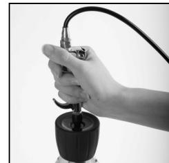
Fig. 8: Repressurize headspace for 5-10 seconds
