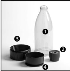
Fig. 1: Shell (1), cap (2), base (3), and booster (4)
