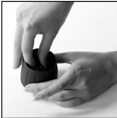
Fig. 10: Grasp valve with fingertips and remove
