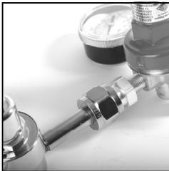
*Fig. 3: Using the CGA-320 adaptor on high-pressure port of existing regulator*
