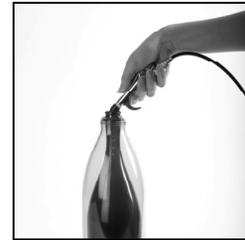
Fig. 6: Purge air from headspace for 3-5 seconds
