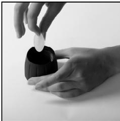
Fig. 11: Press new valve in with fingertips
